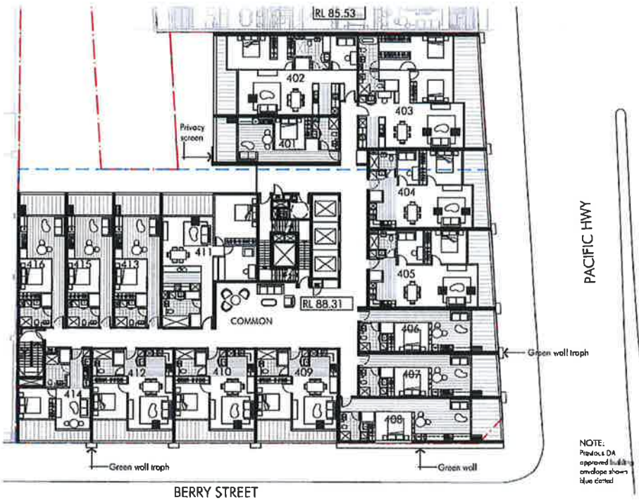
Figure 6 – Example Floor Plate (Level 4)
